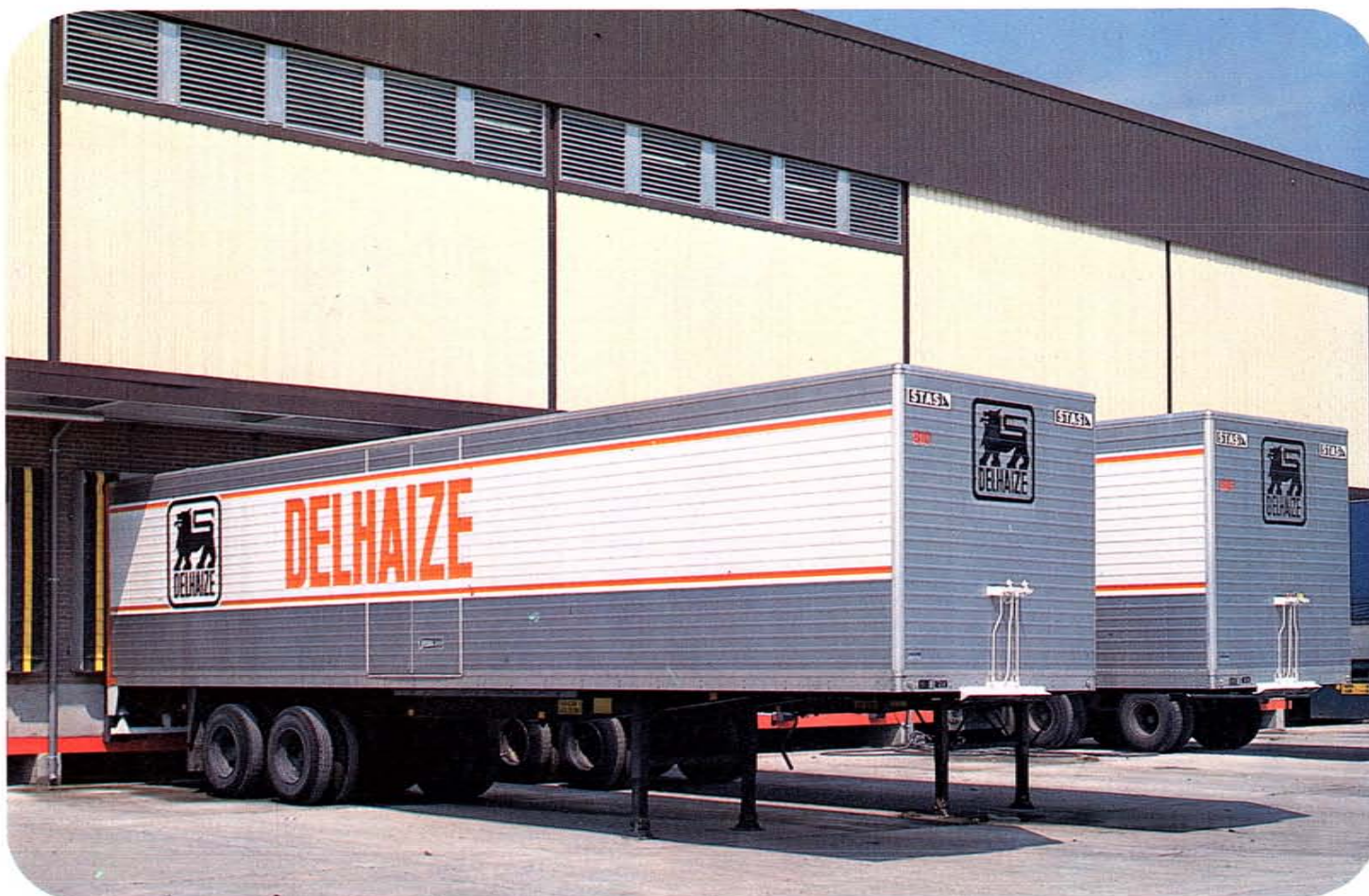
Riveted aluminium semi trailers ALUVAN Semi-remorques ALUVAN en aluminium rivé ALUVAN opleggers in geklonken aluminium
